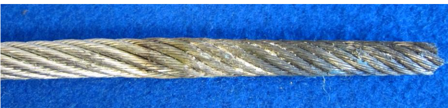
Rope end annealed with a blowpipe and twisted
